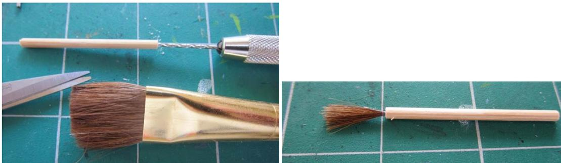
The tiny paintbrush was made from a bamboo skewer with a hold drilled in with a pin vise. Hairs were snipped off a real paintbrush and glued in.
